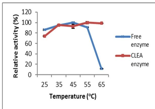
Figure 1. Temperature optimum test for CLEA and free amylase
